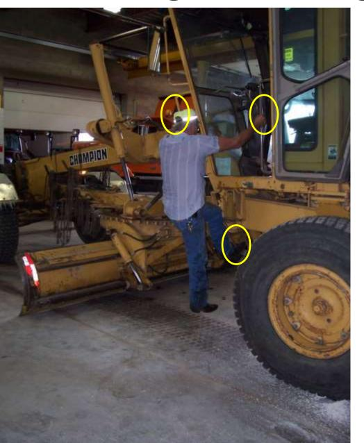
Always keep three points of contact with grader when entering and exiting grader
