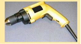
Such tools are often used in areas where there is considerable moisture or wetness. Although the user is *insulated* from the electrical wiring components, water can still enter the tool's housing. Ordinary water is a conductor of electricity. If water contacts the energized parts inside the housing, it provides a path to the outside, bypassing the double insulation. When a person holding a hand tool under these conditions contacts another conductive surface, an electric shock occurs.
