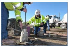
**Pervious Concrete Pavement Study** (LRRB, MnDOT) MnDOT's study of permeability, freeze thaw durability, and maintenance activities at MnROAD and on city streets.
