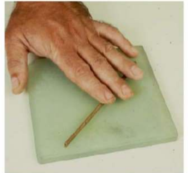
b. Plastic Limit test
