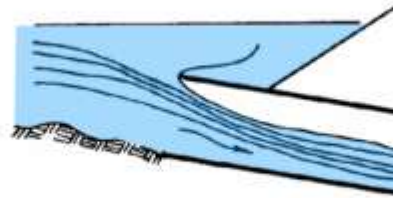
Projecting Square Edge (Applies to Concrete Culverts for non-socket end of the pipe projecting from the fill)
