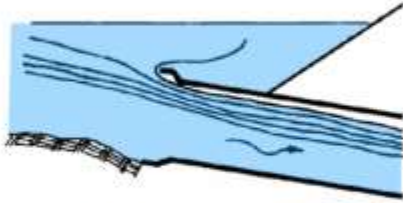
Projecting Groove Edge (Applies only to Concrete Culverts with the socket end projecting from the fill)
