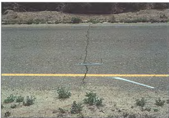
Figure 21: Distress Type ACP 6 High Severity Transverse Cracking
