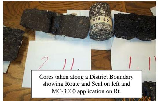
Cores taken along a District Boundary showing Route and Seal on left and MC-3000 application on Rt.
