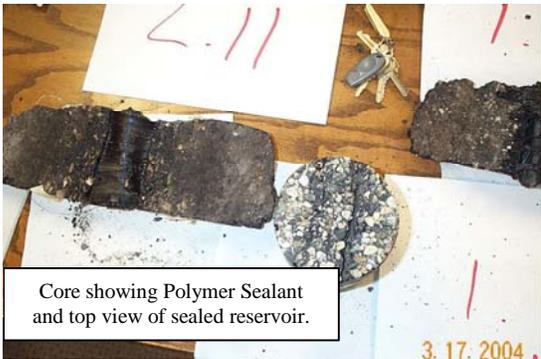
Core showing Polymer Sealant and top view of sealed reservoir.
