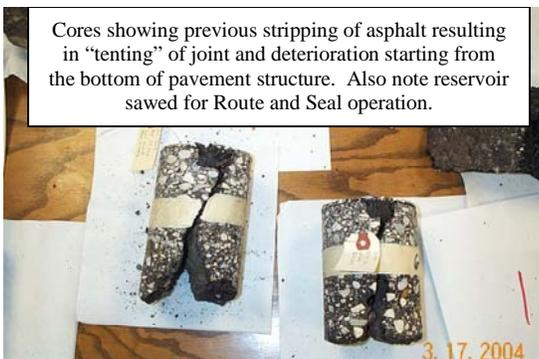
Cores showing previous stripping of asphalt resulting in “tenting” of joint and deterioration starting from the bottom of pavement structure. Also note reservoir sawed for Route and Seal operation.
