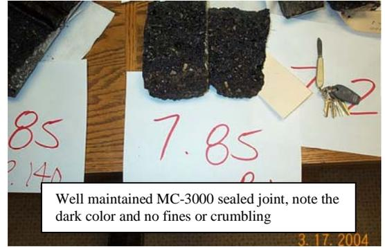
Well maintained MC-3000 sealed joint, note the dark color and no fines or crumbling
