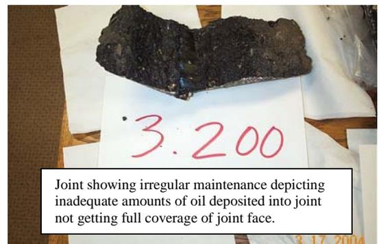
Joint showing irregular maintenance depicting inadequate amounts of oil deposited into joint not getting full coverage of joint face.
