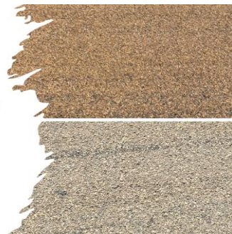
Asphalt Surface Treatment – Natural Aggregate With CRS-2P Emulsion
