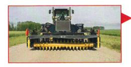
The Grader Mount Sod Mulcher features quick change carbide drum teeth
