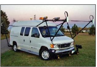
NDDOT Pathways High Speed Inertial Profiler
