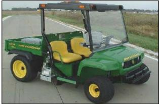
**NDDOT Lightweight Inertial Profiler**
