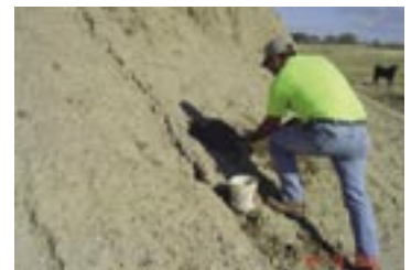
Taking a sample of the binder material from a stockpile.
