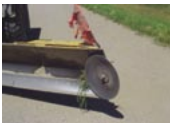
The Gravel Saver disk in place on moldboard.
