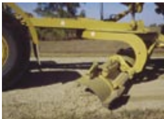
Material loss from toe of moldboard.
