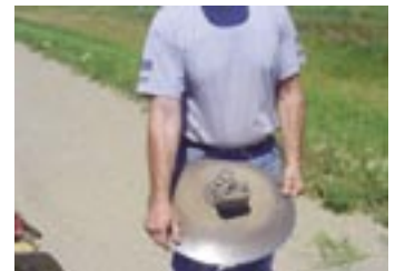
The device has a simple two-bolt mount and is used on either side of the moldboard.
