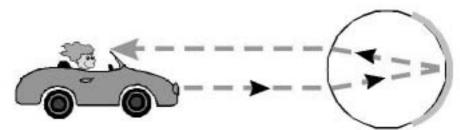
Figure 6. Bead retroreflection
