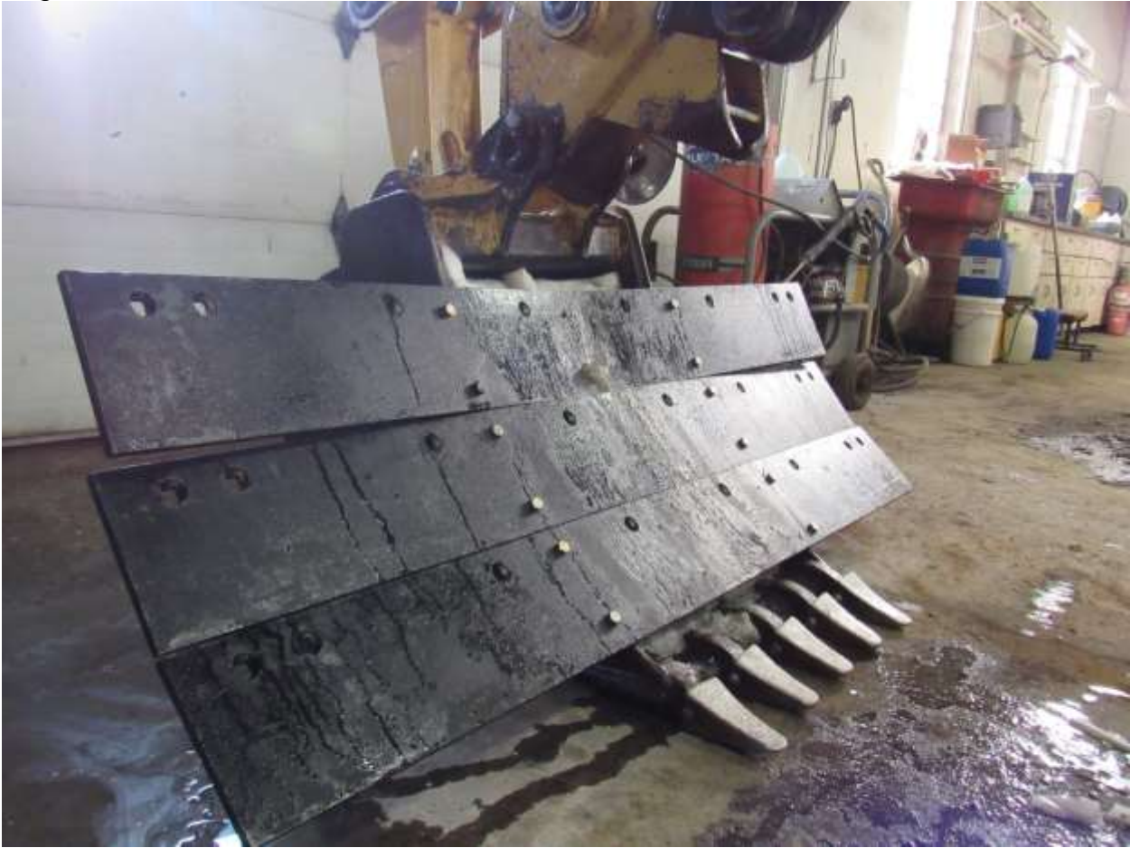
Angle view of snow bank buster attached to backhoe bucket.
