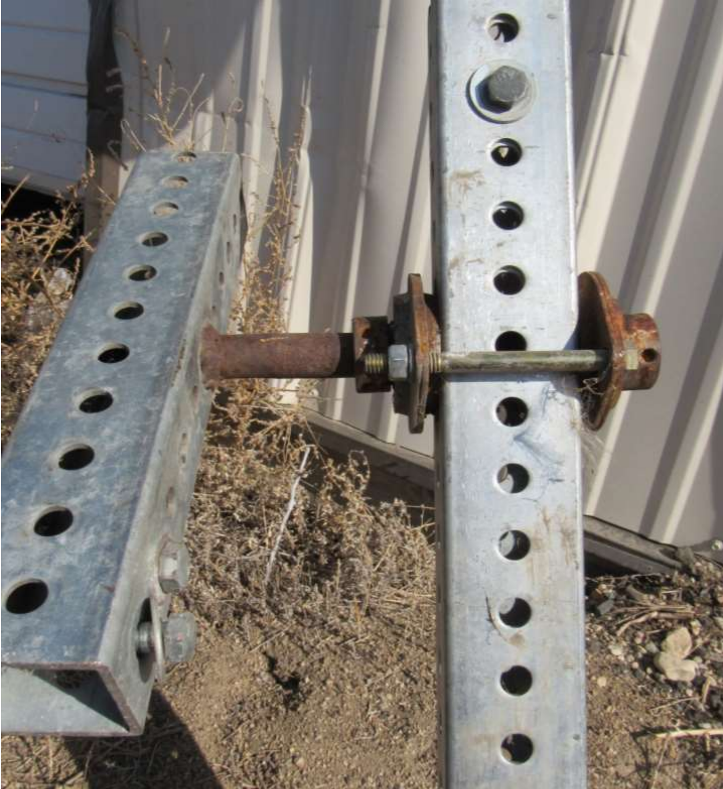
Steel rod inserted and roller bearings mounted on post creating pivot point. Rod welded to bridge mount.
