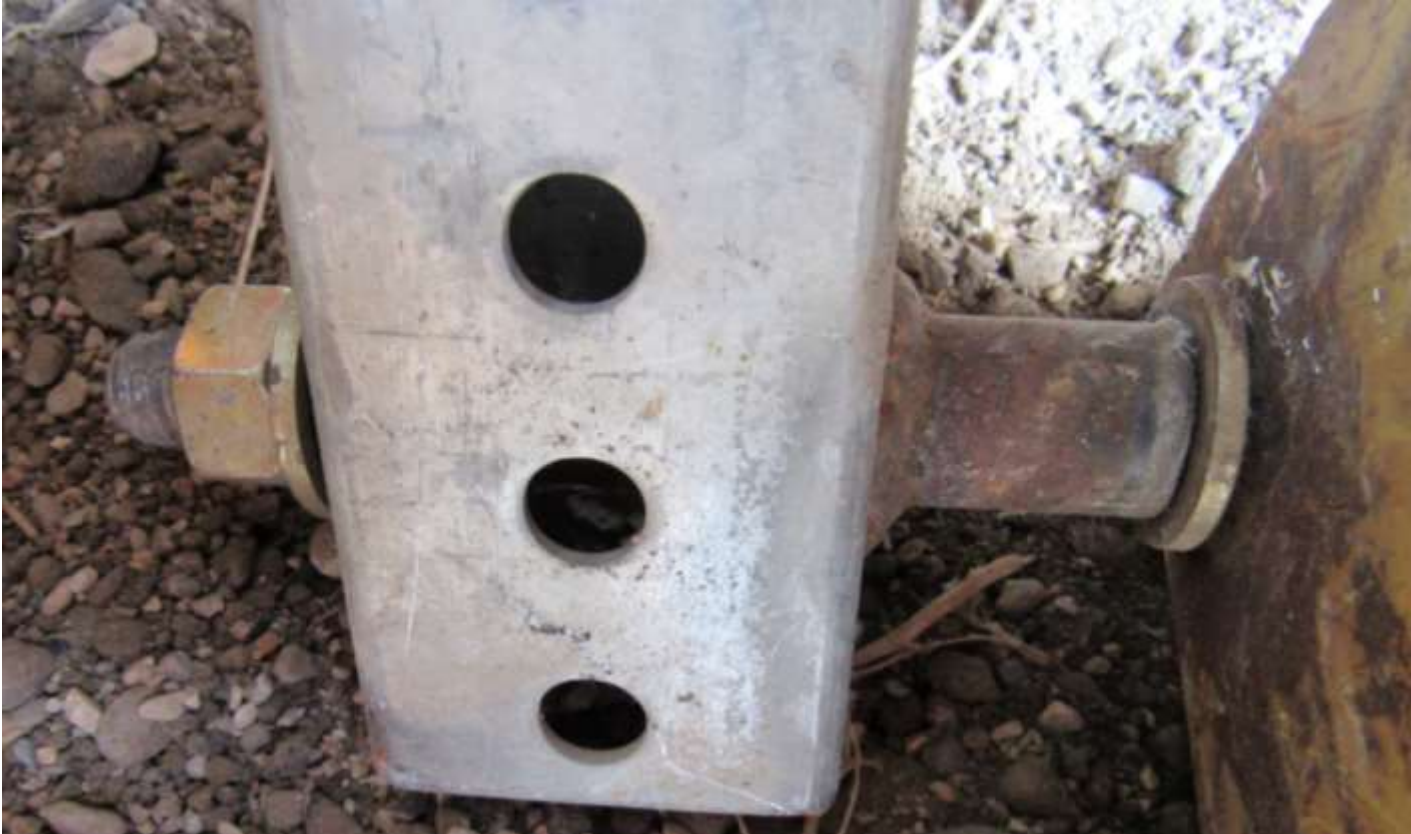
Countweight attaches to post using a sleeved 7-inch long 1/2-inch bolt, washer, nut, creating a pivot point.
