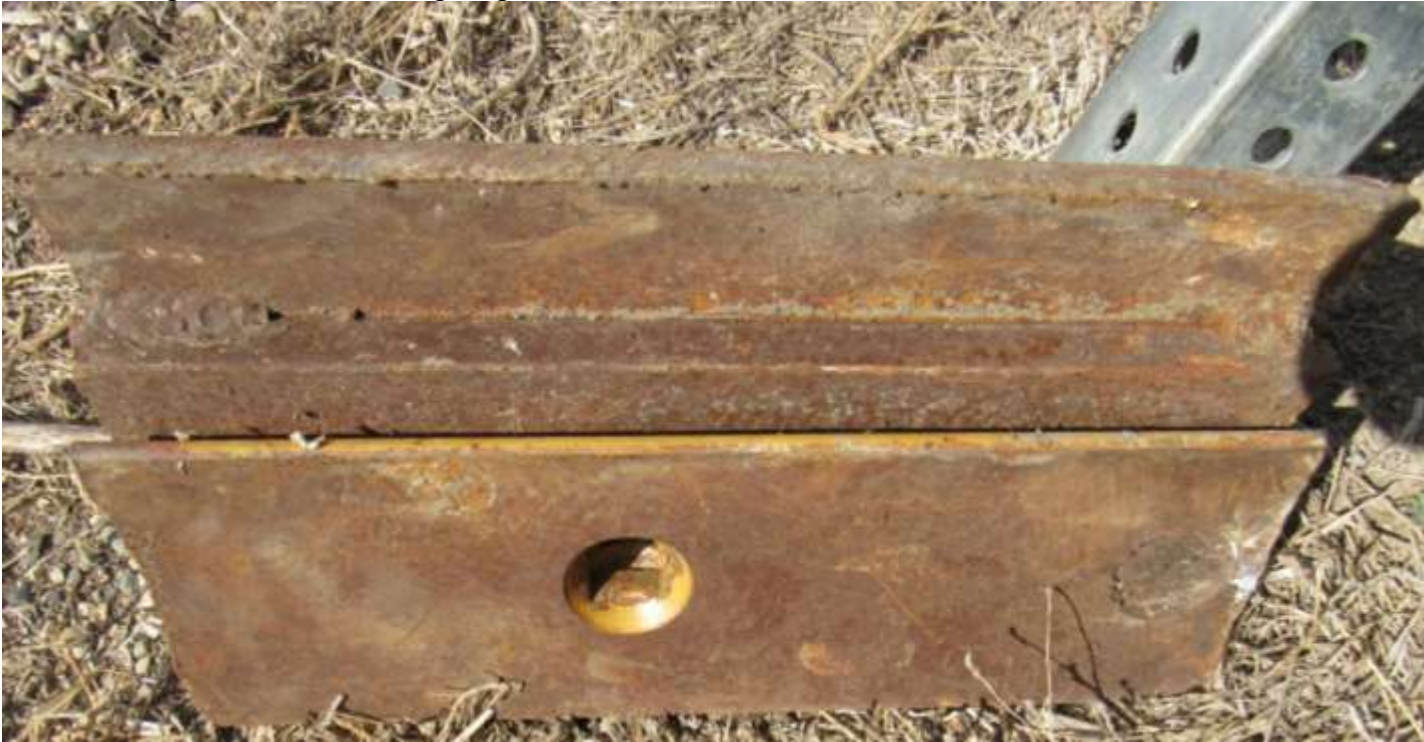
Counterweight – welded cutting edges off a moldboard.
