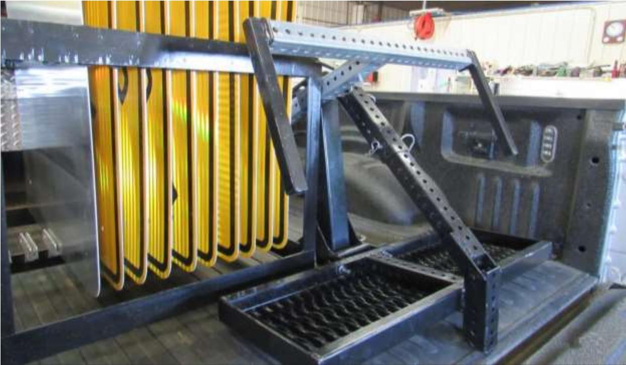
Sign rack – roads signs are easily accessible. No need to climb into pickup box to search through a multitude of signs laying on the bed.
