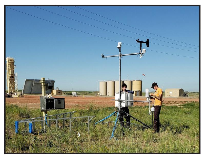
with sub-surface probes provides detailed weather conditions and forecasts along with sub-surface moisture and temperatures to help roadway owners make more refined decisions.
