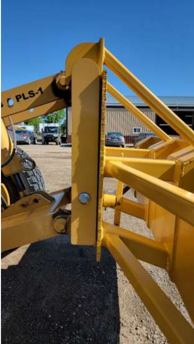
Push-all dozer attached to maintainer
