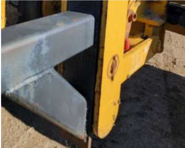
Braces and supports on main base frame
