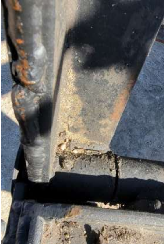
Hinge allows disc frame arm to flex
