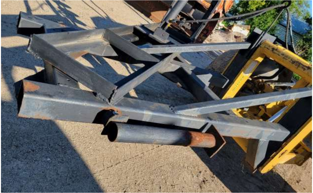
Disc base frame sets on Main frame at 45 degree angle.
