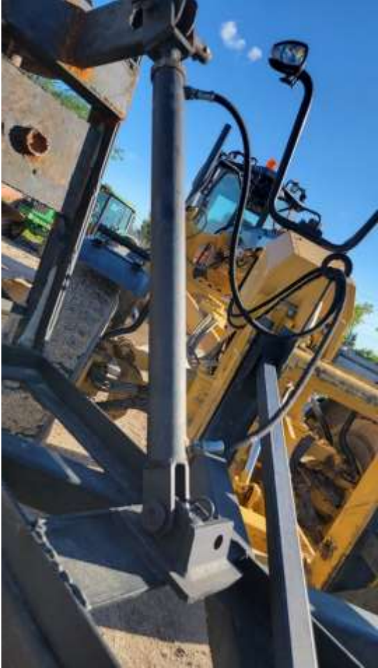
Cylinder attaches to tower and cylinder bracket on disc base frame
