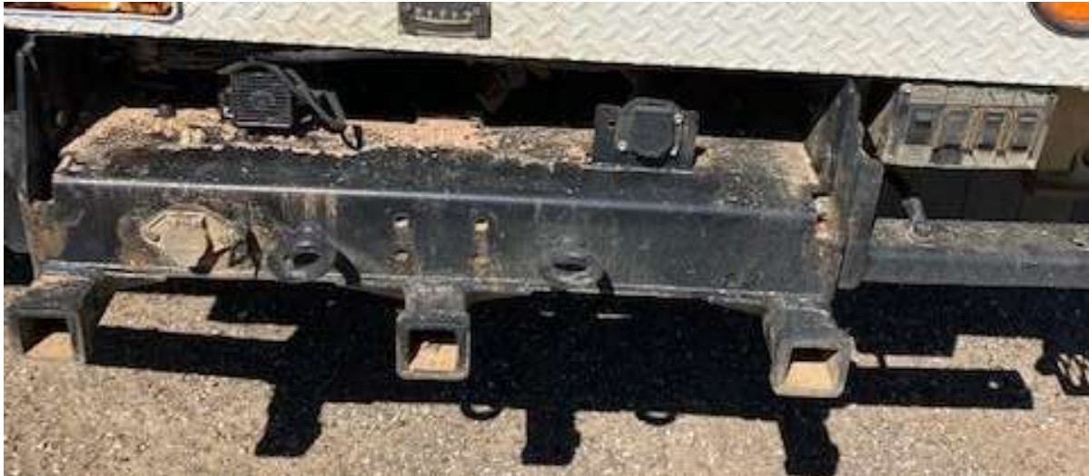
2 receiver tubes welded to hitch on tool truck
