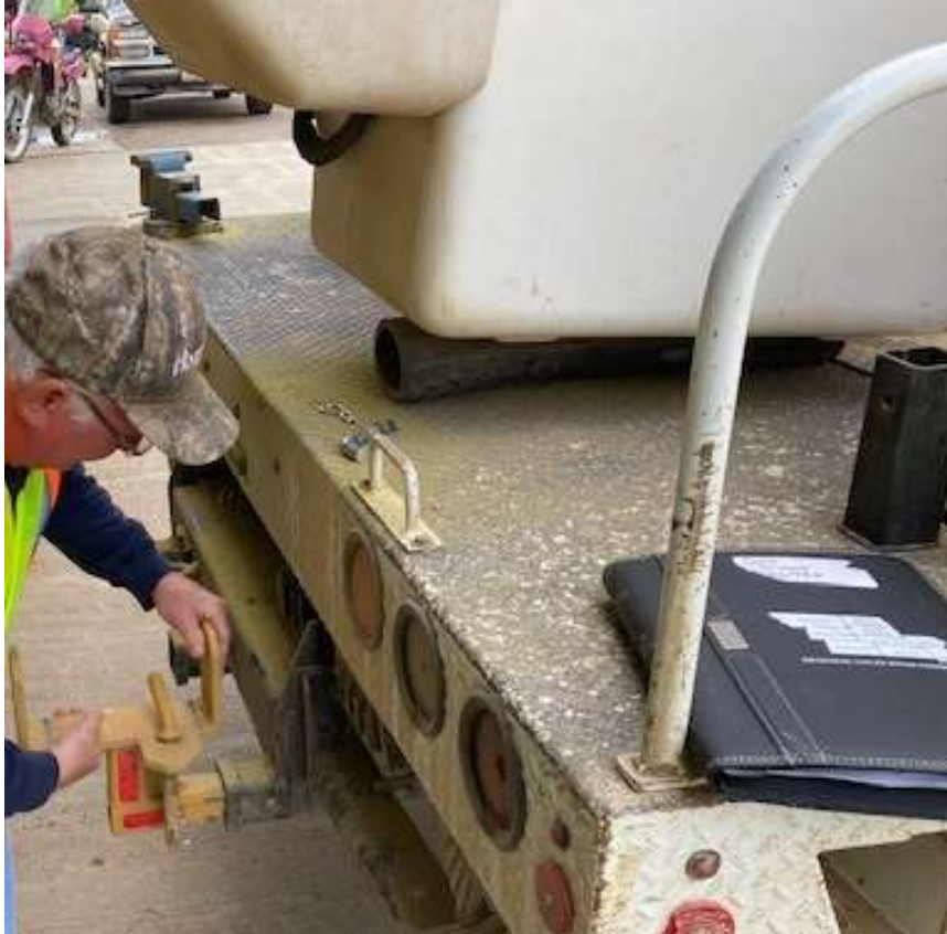
Attach cutting edge carrier to receiver tube. Secure with pins
