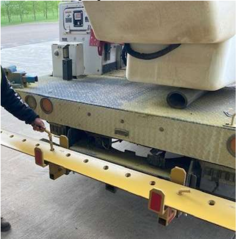
Pins secure cutting edge to carrier
