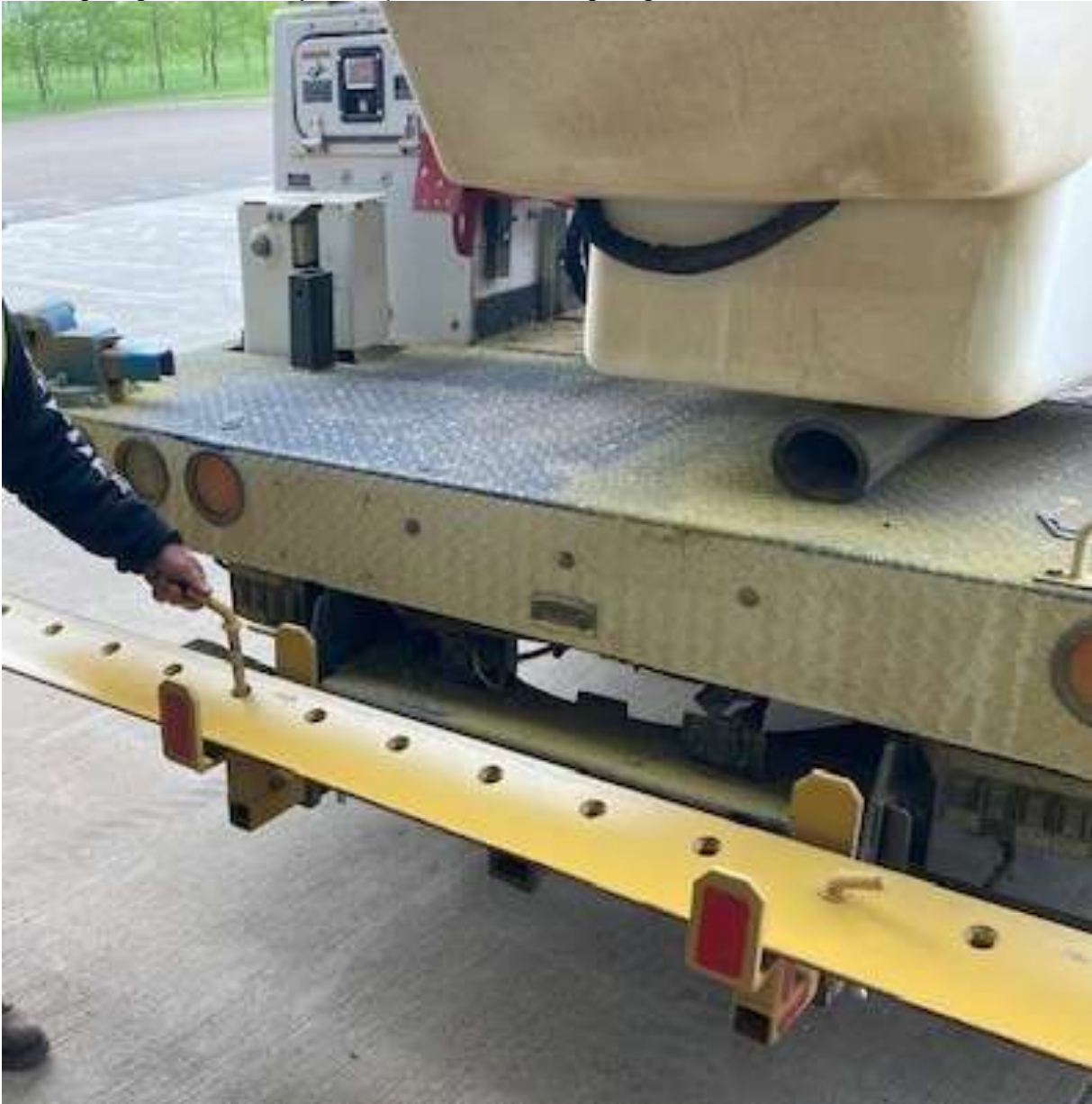
Cutting edges are safely transported on cutting edge carrier mounted on tool truck
