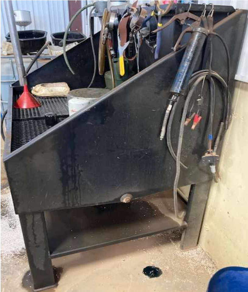
Metal collector table top. Drain plug on side for clean out.
