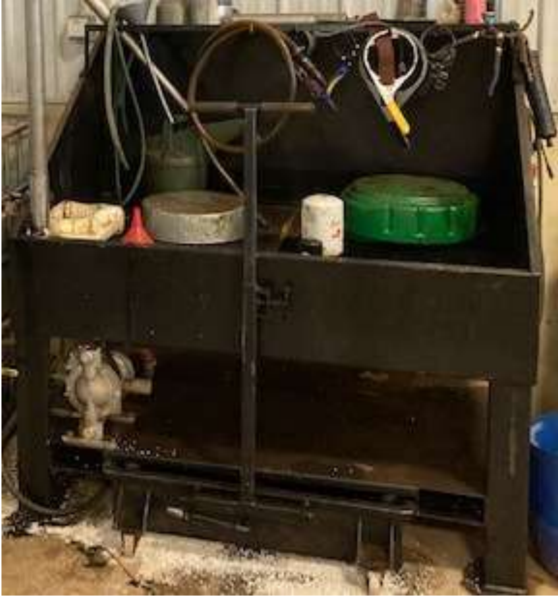
5' x 40" x 36" Stationary oil collection table.
