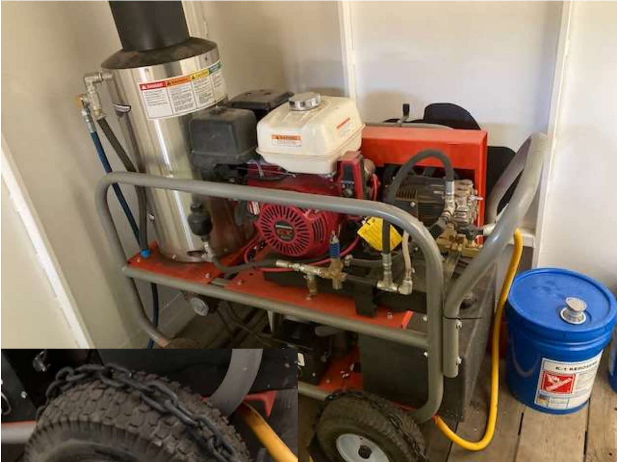
Power washer/water heater unit
