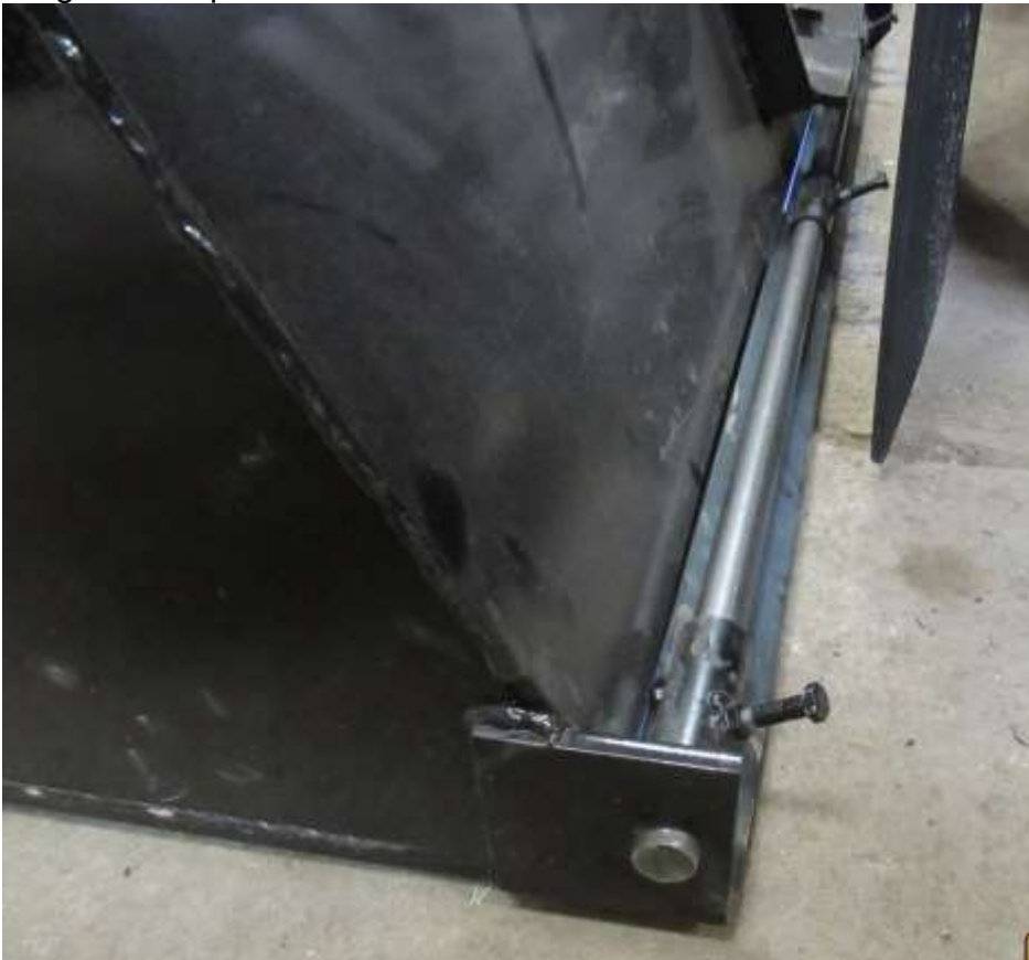
2x3" plates with 1" hole welded on each end of bucket, for 1" round shaft Hinges for flap door
