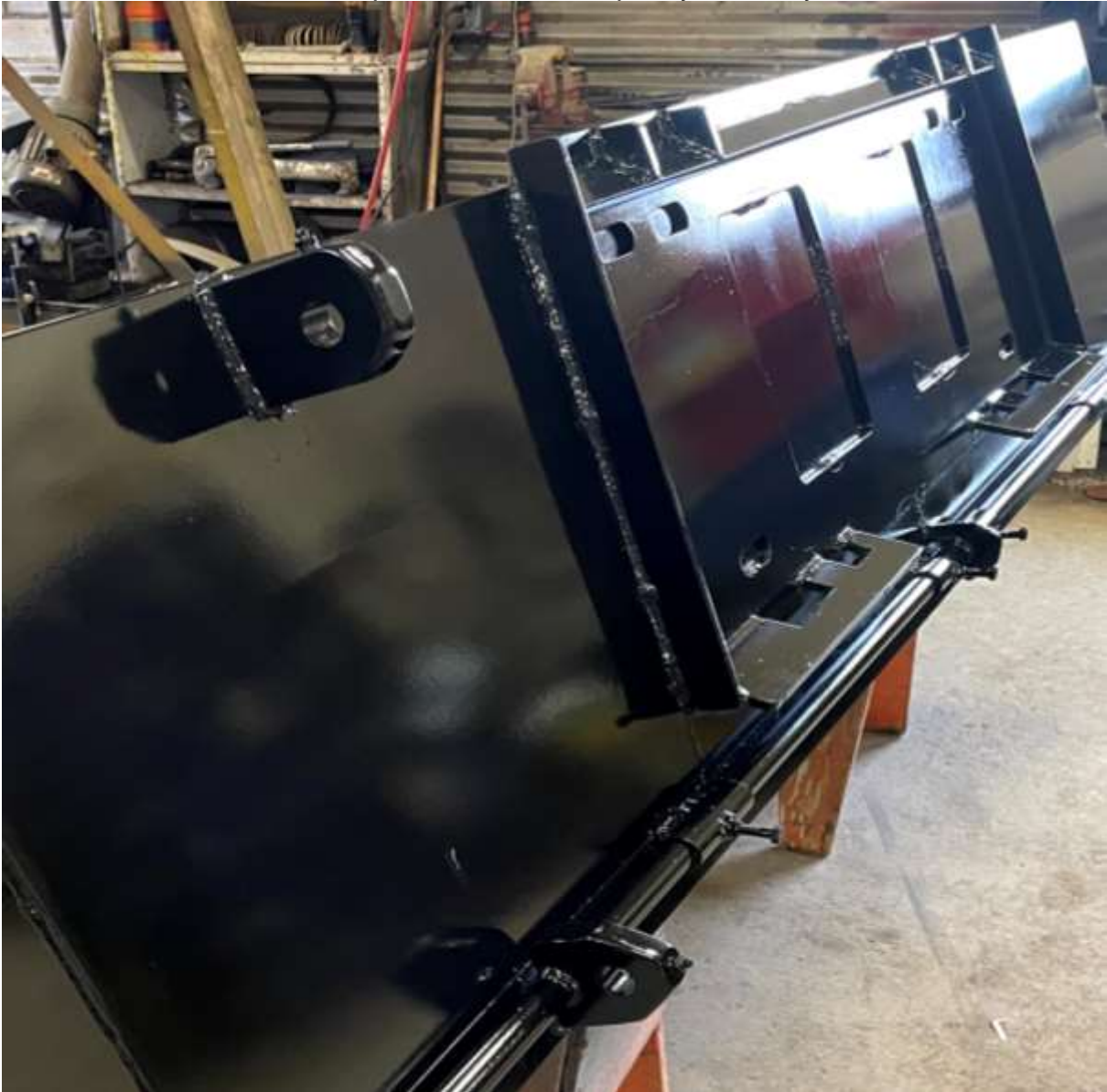
Blank skid-steer attachment plate. Brackets to pin hydraulic cylinder
