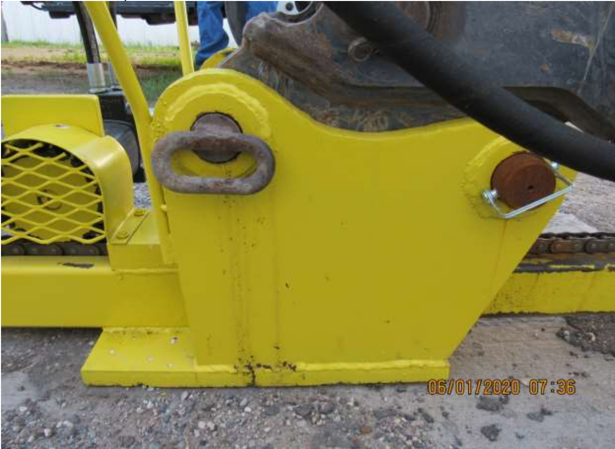
Sideview of steel plate cut to fit backhoe.
