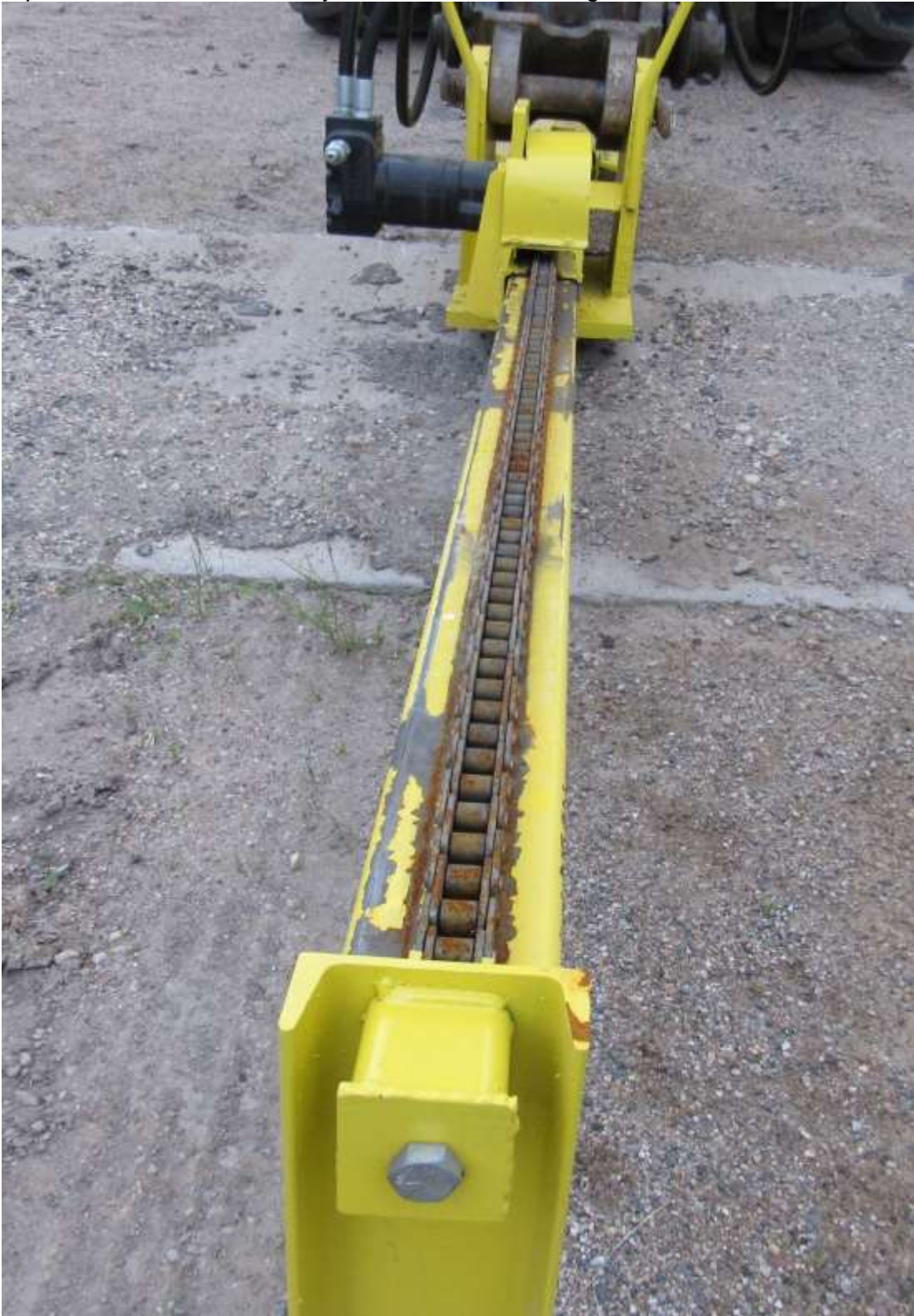
Pipe cleaner extended away from backhoe. Bolt tightener on the end.
