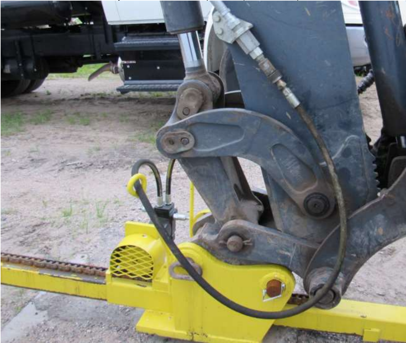
Quick attach to backhoe, hydraulics, 18-tooth sprocket (under cover).
