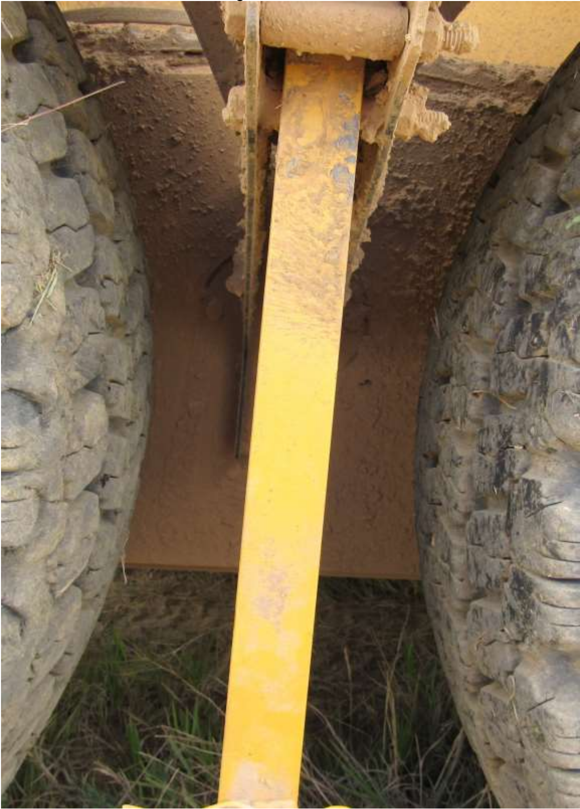
Tube with inserted bolt act as hinge. 19-inch flat iron.
