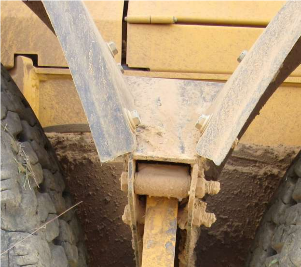
Close up of fender bracket, bolts and tube.
