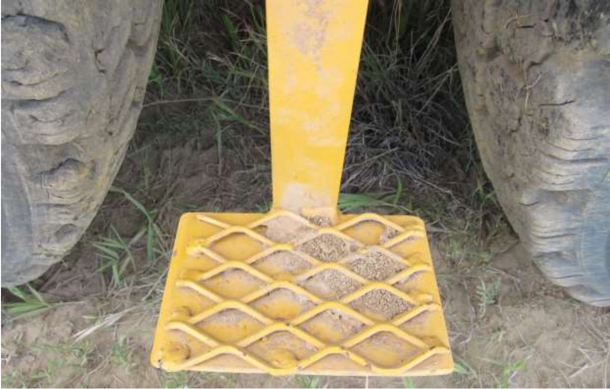
Expanded metal tread plate on step for safety.
