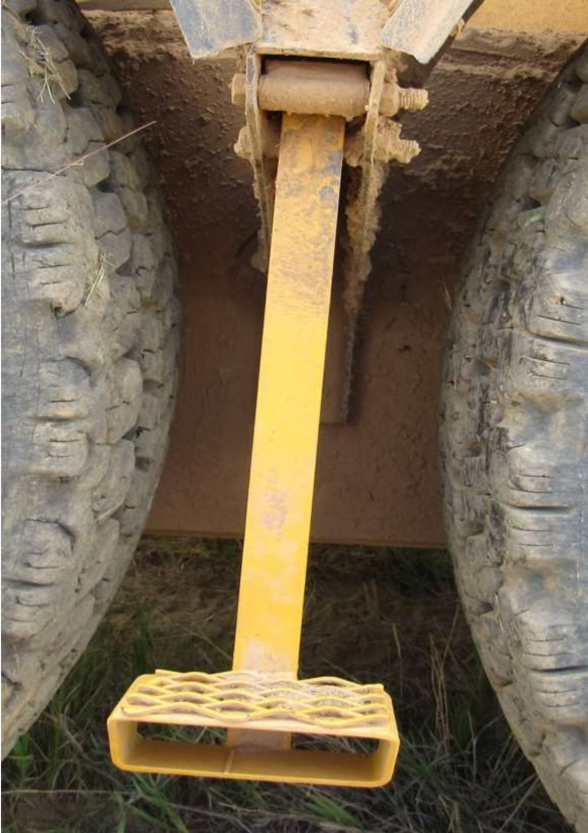
Step attaches to fender bracket between tandem axle.
