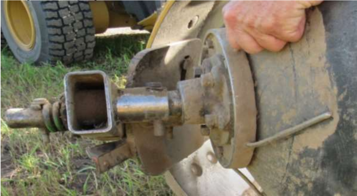
Flexing action of spring-load arm.
