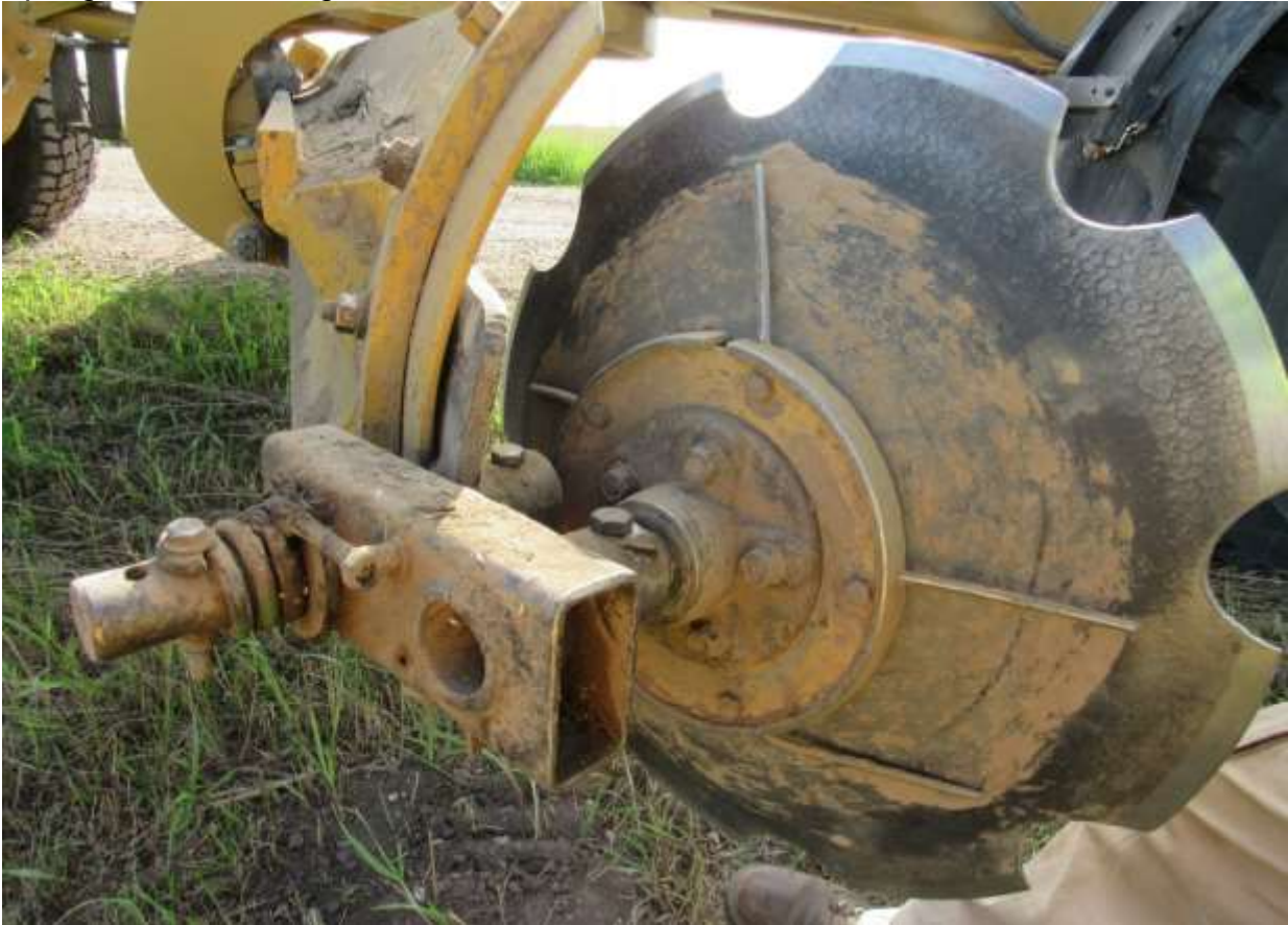
Spring-load arm with gravel saver disc attached.
