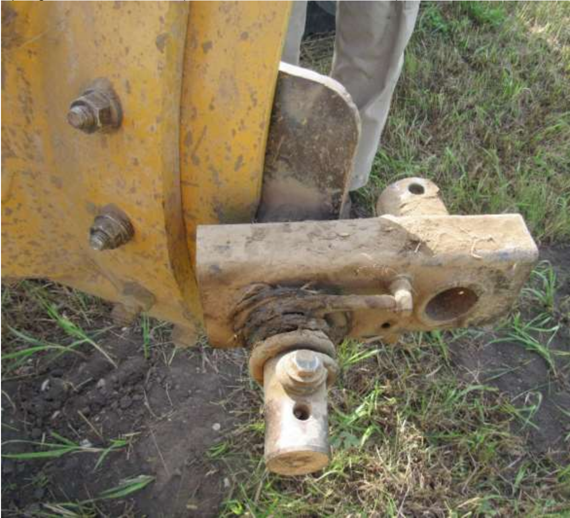
Spring-load arm attached (view from back side of bracket).
