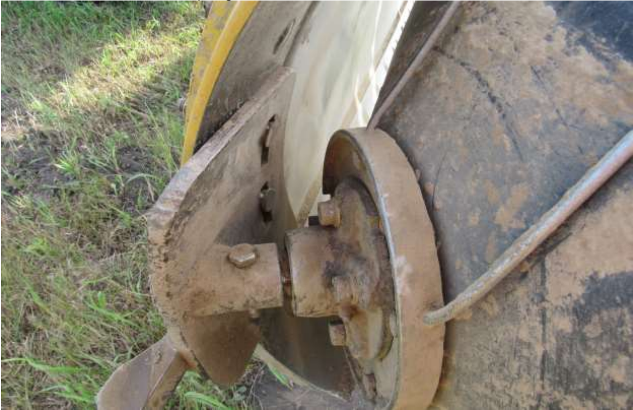
Gravel saver disc without Spring Load Arm Enhancement
