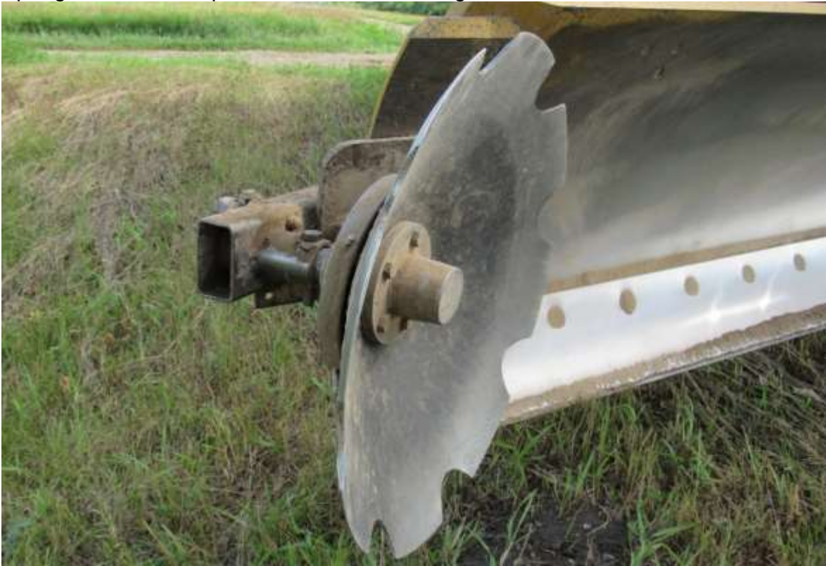
Spring-load arm rest prevents disc from flexing to far down.
