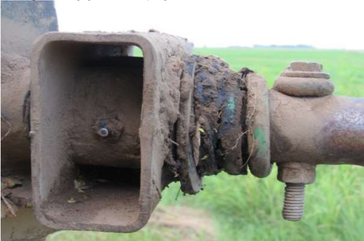
Rectangular tubing, grease zerk, spring tooth, 3/8-inch bolt, and 1 3/4-inch shaft.
