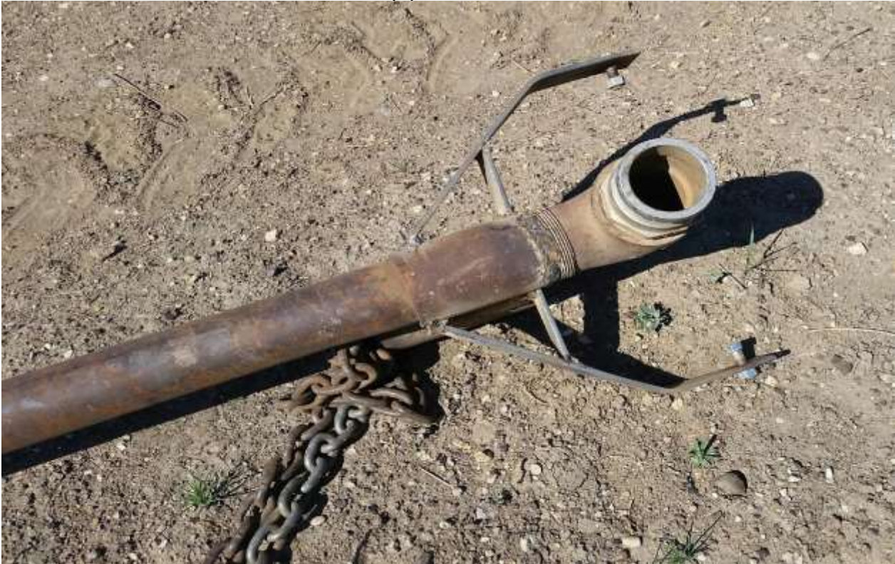
Flat iron brackets and chain welded to pipe.
