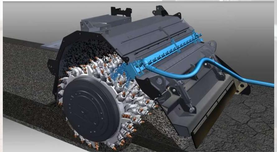
Substantial advances in drum and housing design to maximize the mixing action of the reclaimer
