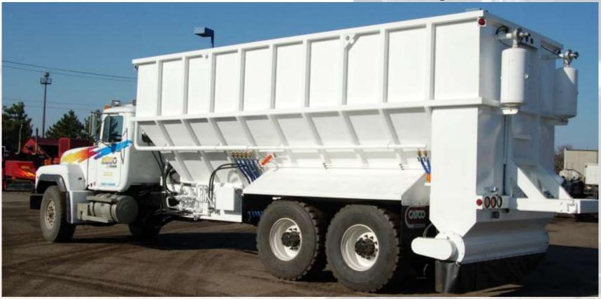
Material application rate controlled by onboard computer that is constantly collecting GPS and ground radar data to apply the proper amount of Portland cement regardless of conditions or the ground speed of the spreader
