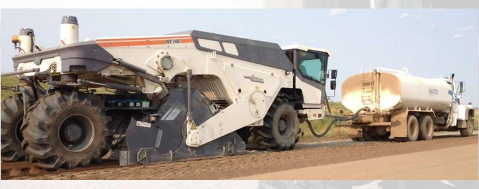
Mass flow meter tied to centralized computer that controls the incorporation rate of water, leading to proper hydration of the cement throughout the stabilized layer
