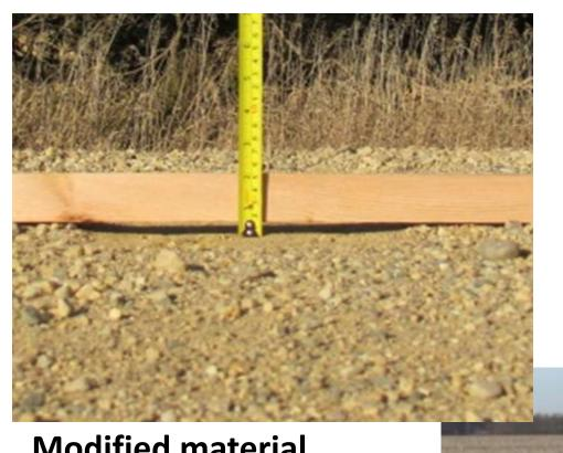
Substandard gravel loosens in 31 days. Loose aggregate (or float) is 1 ¼ to 1 ½ inches between the wheel paths.
