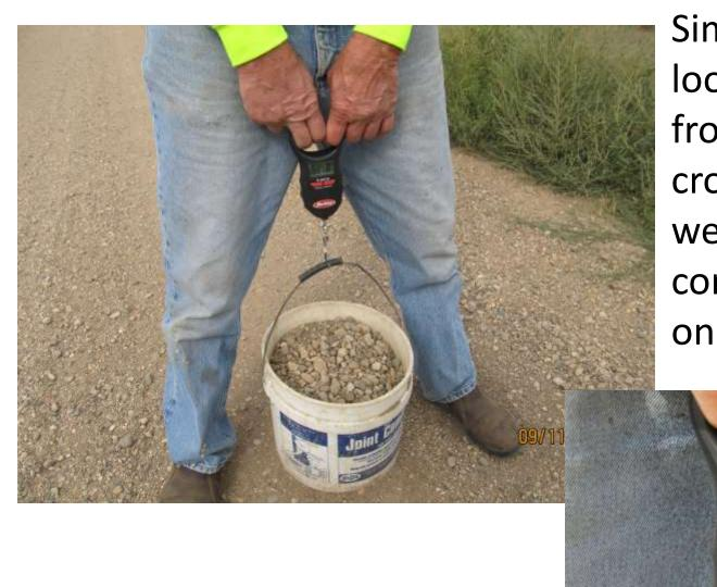
Simply remove loose aggregate from a 10 inch cross section, weigh it and convert that to a one-mile section
