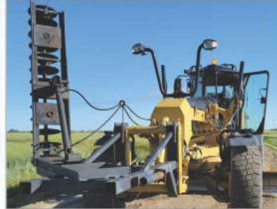
**Grader Mounted Sod Mulcher**
