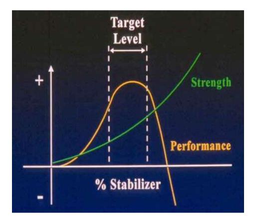
The purpose of the mix design procedure is to select the correct amount of stabilizer that most closely balances both strength AND performance for the roadway materials!
