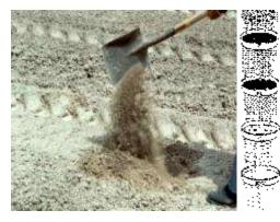
A common gradation requirement is for 100 percent to pass a 3-inch sieve, a minimum of 95 percent to pass a 2-inch sieve, and a minimum of 55 percent to pass a
