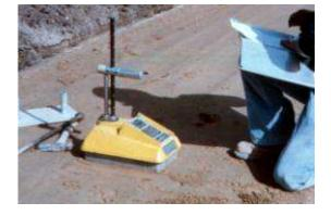
A common density requirement is to be between 96 and 98 percent of the established laboratory standard Proctor density (ASTM D558). Moisture
