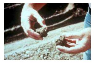
A common moisture requirement is to be within 2 percent of the laboratory established optimum moisture content (ASTM D558).
