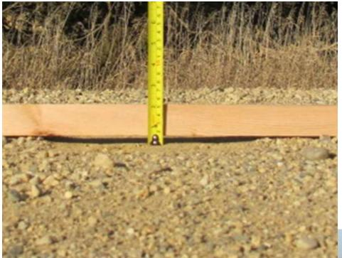
Substandard gravel loosens in 31 days. Loose aggregate (or float) is 1¼ to 1½ inches between the wheel paths.
