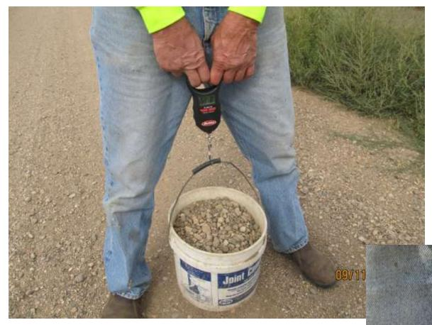
Simply remove loose aggregate from a 10 inch cross section, weigh it and convert that to a one-mile section
