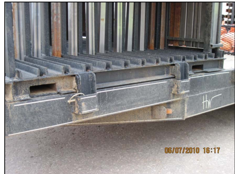
Quick release pins and holes for forklift forks
