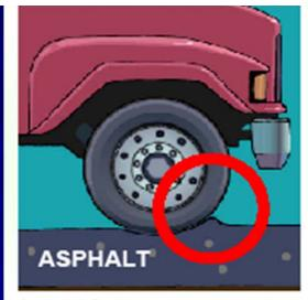
Asphalt deflection causes energy to be absorbed ... and more fuel to be used.
