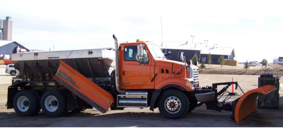
The last five trucks purchased by Pennington County have the Kabota Quick Attach System. This system allows the trucks to be utilized as a plow and sander, dump truck or 5<sup>th</sup> wheel tractor.
