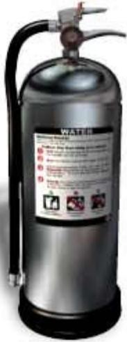
Water is one of the most commonly used extinguishing agents for type A fires. You can recognize an APW by its large silver container. They are filled about two-thirds of the way with ordinary water, then pressurized with air. In some cases, detergents are added to the water to produce a foam. They stand about two to three feet tall and weigh approximately 25 pounds when full.
