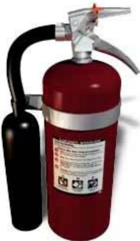
This type of extinguisher is filled with Carbon Dioxide (CO<sub>2</sub>), a non-flammable gas under extreme pressure. These extinguishers put out fires by displacing oxygen, or taking away the oxygen element of the fire triangle. Because of its high pressure, when you use this extinguisher pieces of dry ice shoot from the horn, which also has a cooling effect on the fire.
