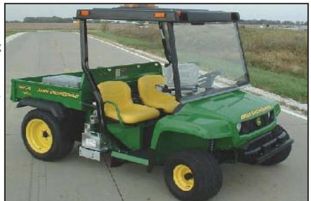
NDDOT Lightweight Inertial Profiler
