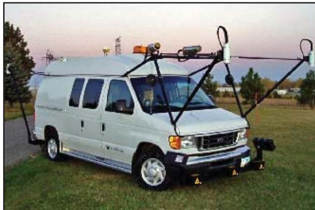
NDDOT Pathways High Speed Inertial Profiler
