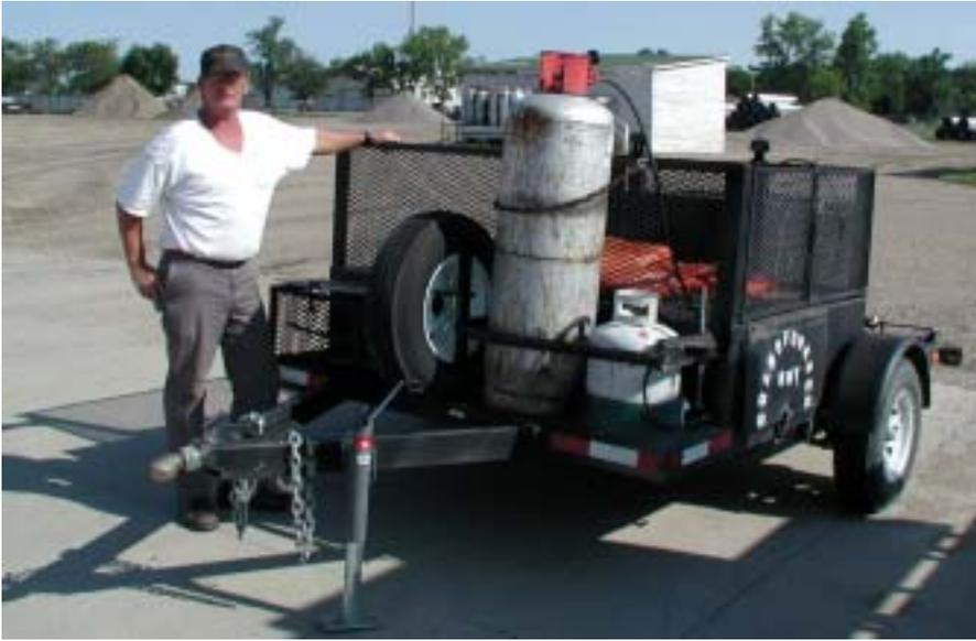
Gary Johnson with the hot box for asphalt mix
